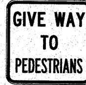
Figure 2 – GIVE WAY TO PEDESTRIANS (R2-10) sign
